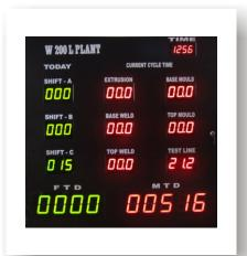
Ajinkya offers production displays to show information like production count, turn around time, shift count, total production, efficiency, information display systems, production display systems etc. as per user requirement. These displays are also termed as Andon displays. These production displays are custom built to suit user requirement.
