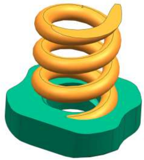
TACK HEAD (MATERIAL : PEEK) SPRING INSERT MOULDING) PART SIZE: 4 x 4 x 4 mm
