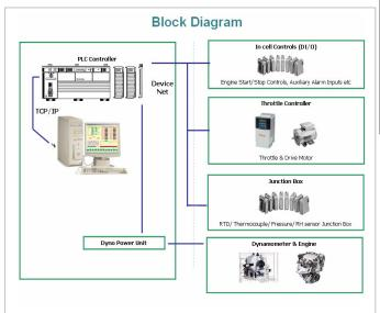
In above block diagram, Integrated Engine Dynamometer is described in two sections: Control consol and In-cell controls.
