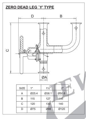
The GMP loop valves can be utilized to virtually eliminate dead legs in the design of point of use outlets in a typical WFI distribution loop. The process fluid flows through the valve body.
