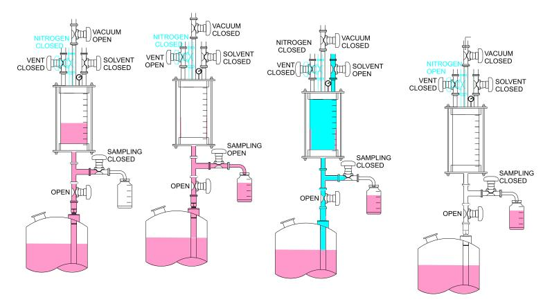
Extracts a liquid sample from reactors and vessels via a dip pipe. Sample is representative, fixed volume and cannot overflow the sample bottle.
