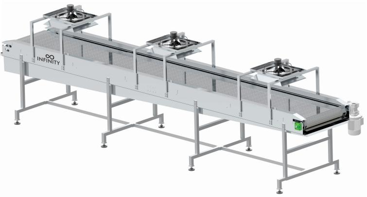
Wire mesh belt conveyors can be used in a variety of conditions to conveyor hot, cold, or oily products in oven, cooling, carrying cold items from a freezer, hot food items or other special conditions. A variety of belt types can be used depending on the application. It's designed to interface with existing conveyor systems and is custom engineered from standard components.
