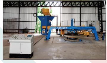
**CAP** Series Machines from Apollo Hawkeye Pedershaab are dry cast machine for manufacturing almost any type of high quality concrete products.
