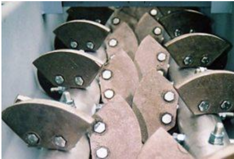
Replaceable blades of Pug Mill Ash conditioner design
