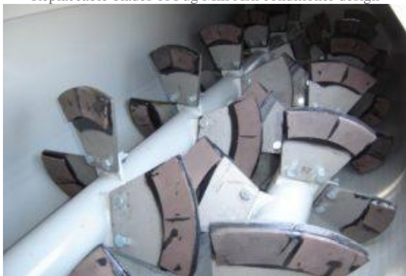
Replaceable blades of Pug Mill Ash conditioner design
