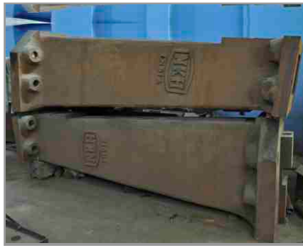
Raw Casting of Columns
