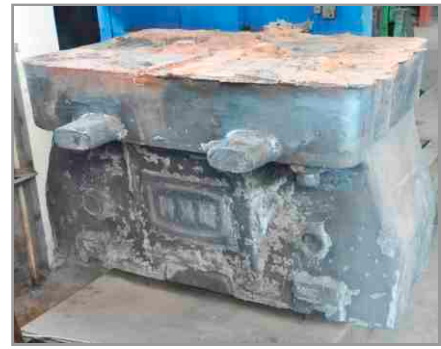
Raw Casting of Anvil Block
