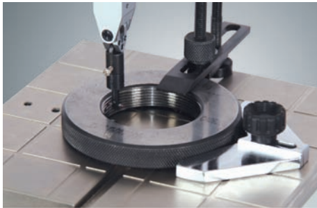
Cy. Measurement of effective diameter by using single arm measuring attachment & Precision Ruby T-Shape styli
