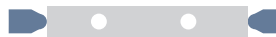
Gauge block / Length Bar measurement by using a pair of ball anvils
