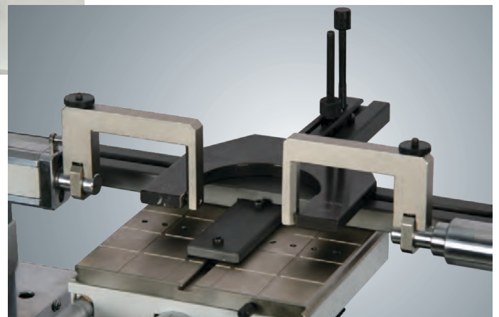
Snap Gauge (below 300 mm) measurement : Hold on snap gauge holding attachment
