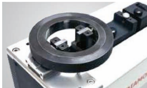
Measurement of Internal Diameter
