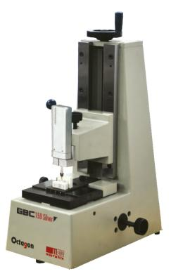
GBC 150 Silver Gauge block comparator with Heidenhain Optical Incremental length gauge of long measuring range 20 mm, resolution 0.01  $\mu$ m and consistently high accuracy  $\pm 0.03\mu$ m at top side and bottom one with the high precision inductive probe.
