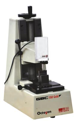
Octagon GBC 150 Gold\* and GBC 150 Silver\* are precision gauge block measuring systems with most advanced feature of longer comparison range of 20mm. Both Gauge block comparators used for precision gauge block measurement, designed with two electrical high resolution length indicators (summeasurements) as recommended in ISO 3650. Octagon Gauge block comparators
