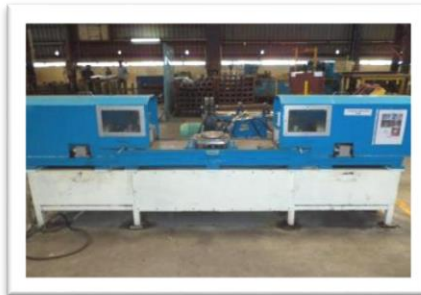
FLANGE DRILLING SPM
