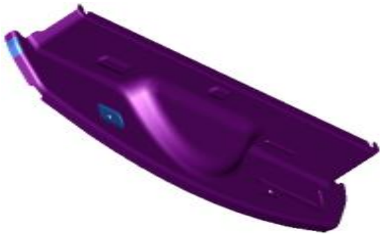
REINFORCEMENT-U/B RR CR SILL LWR
