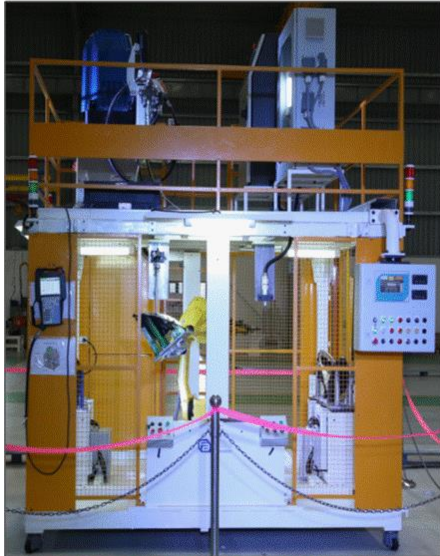
o Plasma Heating and Gluing Robotic Cell
