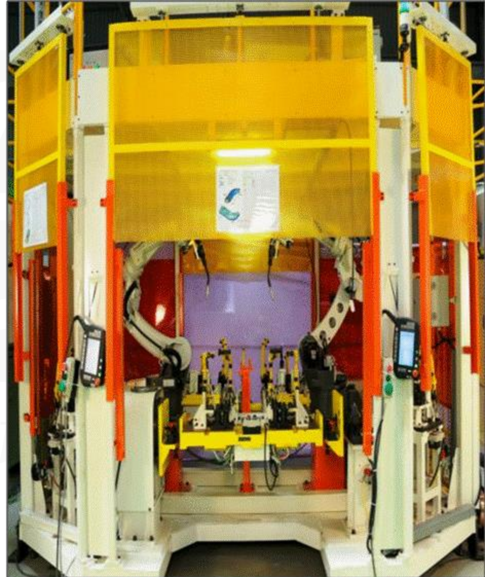
o MIG Welding Robotic Cell
