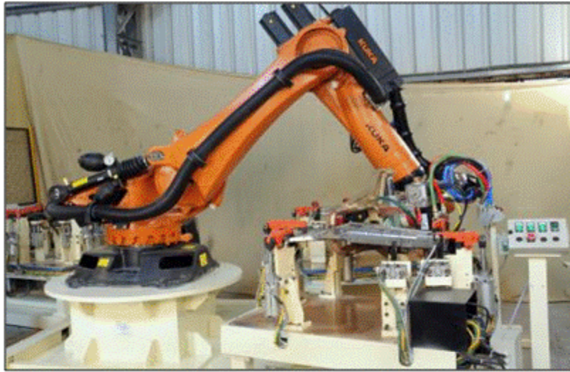
○ Spot welding Robotic Cell
