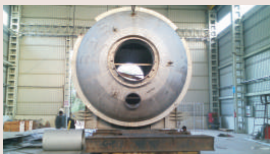
De-SuperHeater with Tube Bundle Assembly Size: 4.8m Dia X 5m Length
