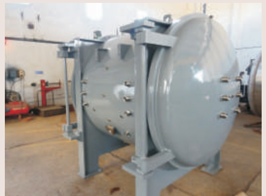
Jacketed Vacuum Chamber with Both Side Doors & Hinge Assembly
