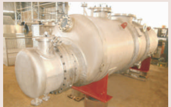
Re-Boiler Kettle with U Tube Bundle for Chemical Plant
