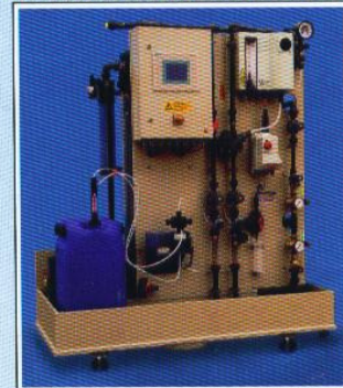
For Chlorination of Water in Cooling Towers
