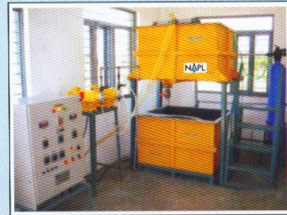
Unique Onsite Hypochlorite Generator.
