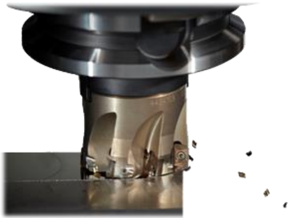
Cast Iron Machining
