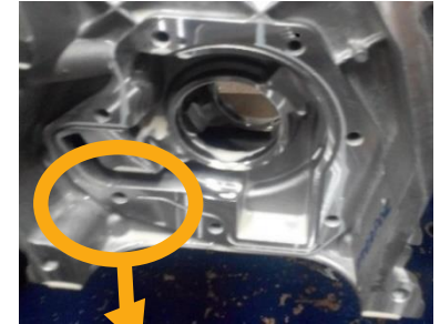
Face and Side wall Milling
